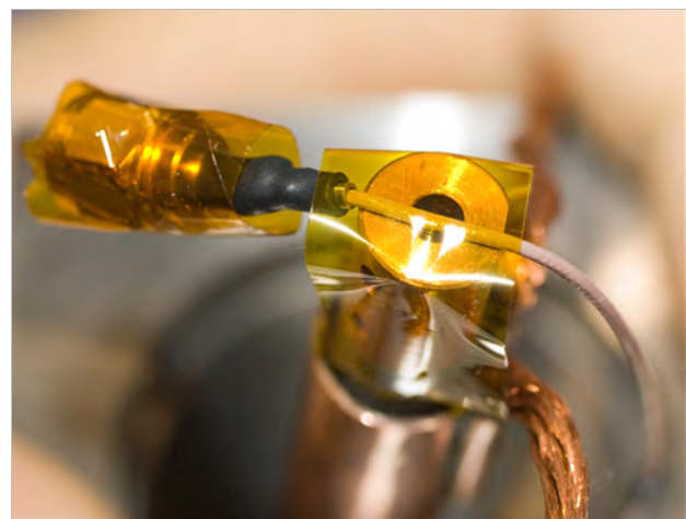
FIGURE 5-11 Left: Securing the planarization assembly to the probe arm base; Right: Taping the cable to the probe arm
