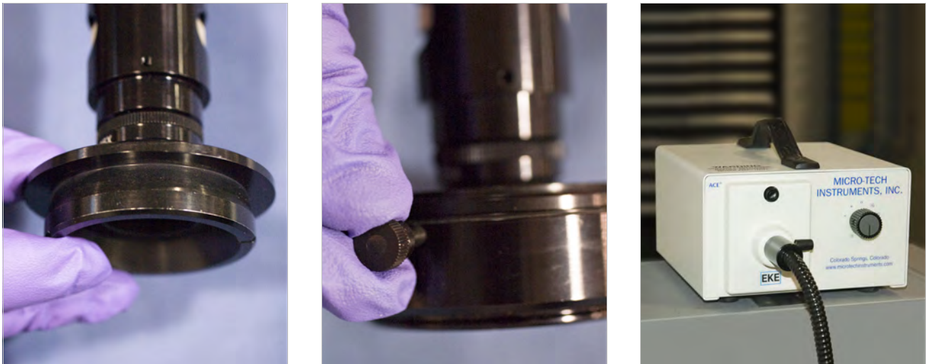
FIGURE 3-24 Left: Installing the ring light onto the adapter; Middle: Tighten the ring light thumbscrews; Right: Fiber optic cable attached to the light source
