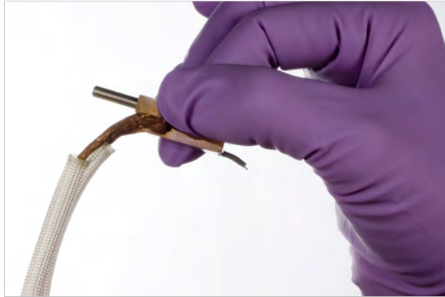
FIGURE 3-39 Proper handling of a microwave probe
