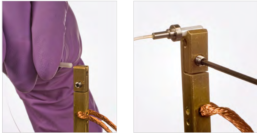
FIGURE 5-21 Left: Inserting the optical fiber tip into the opening in the probe mount; Right: Securing the optical fiber tip by tightening the M3 screw
