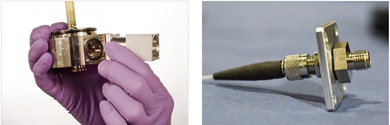
FIGURE 5-19 Left: Attaching the feedthrough extension to the probe arm base; Right: The nut between the cable and the flange—SMA style shown
