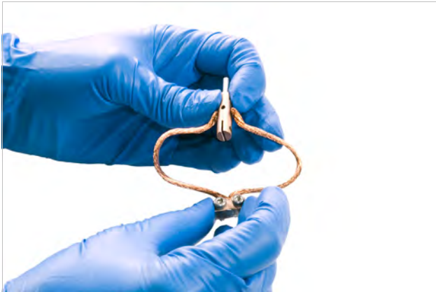
FIGURE 3-32 Left: To install the probe mount, bend the probe mount braids; Right: Apply grease to the end of the dowel
