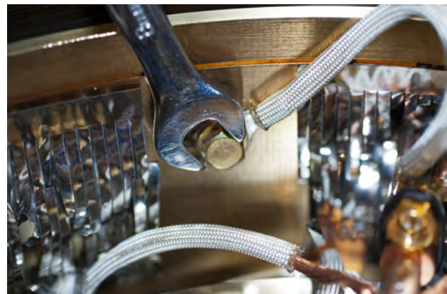
FIGURE 5-4 Left: Slide the spade lug under the hex screw head and washer; Right: Tighten the hex screw
