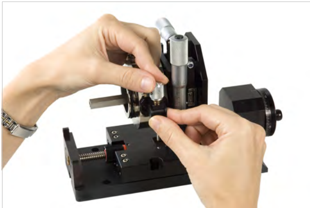
FIGURE 5-24 Left: Thread the shaft through its mounting hole; Right: Attach the planarization assembly to the probe arm base
