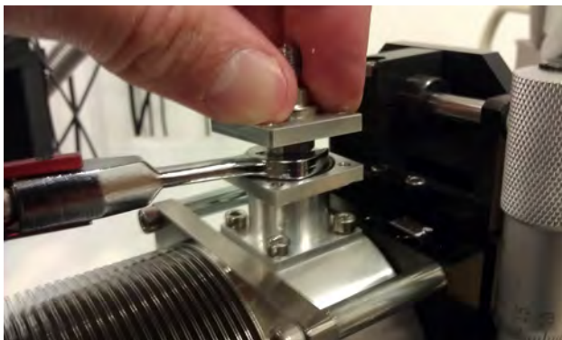
FIGURE 5-17 Left: Rotate the feedthrough assembly into position and retighten the connection; Right: The off-centered position on the cable feedthrough assembly
