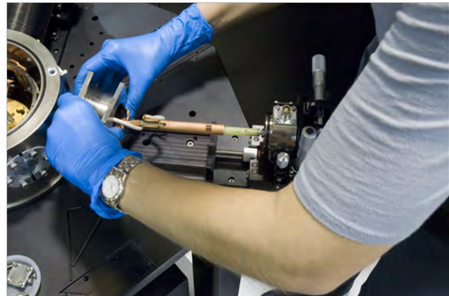
FIGURE 5-8 Left: Remove the four horizontal screws that attach the bellows to the z-axis stage; Right: Compress the bellows to remove it from the probe arm
