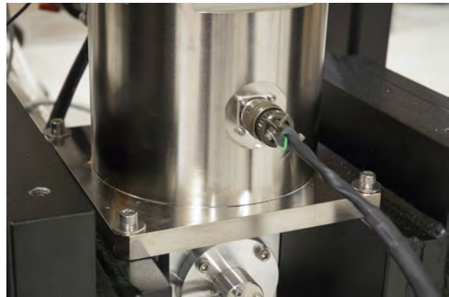
FIGURE 3-19 Left: Cable connection point at the bottom of the vacuum chamber for the sample and radiation shield thermometry; Right: Cable connection point at the side of the vacuum chamber shroud
