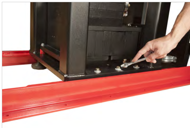
FIGURE 3-8 Removing the cross braces
