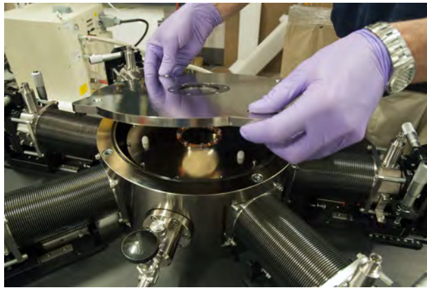
FIGURE 4-3 Probe station vacuum chamber lid removal
