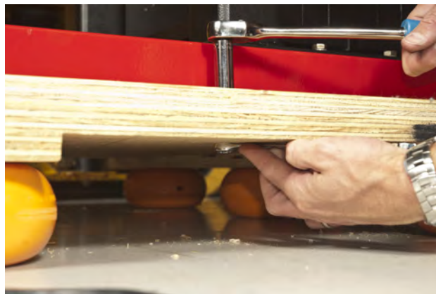
FIGURE 3-6 Remove the bolts attaching the red, horizontal cross braces to the crate base
