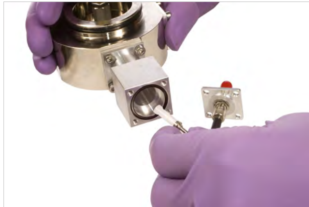
FIGURE 5-20 Insert the optical fiber tip into the feedthrough extension
