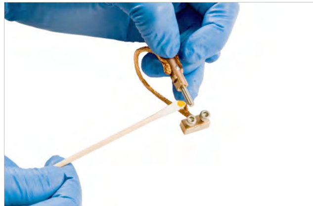
FIGURE 3-32 Left: To install the probe mount, bend the probe mount braids; Right: Apply grease to the end of the dowel
