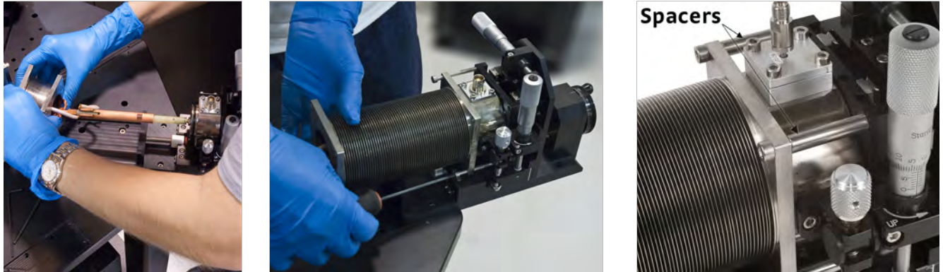
FIGURE 5-12 Left: Placing the bellows onto the probe arm base; Middle: Attach the bellows to the z-axis stage; Right: Spacers between the bellows and the z-axis stage
