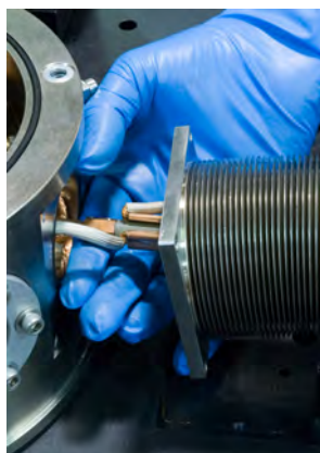
FIGURE 5-2 Left: Prepare the o-ring and groove; Middle: Guide the cable and probe arm through the arm port; Right: Secure the stage to the table
