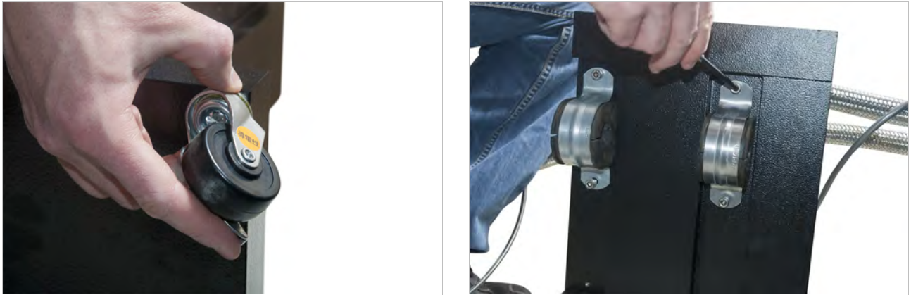
FIGURE 3-17 Left: Finger tighten the locking wheel on the bottom of the helium line isolator; Right: Remove the hose clamps on both sides of the helium line isolator
