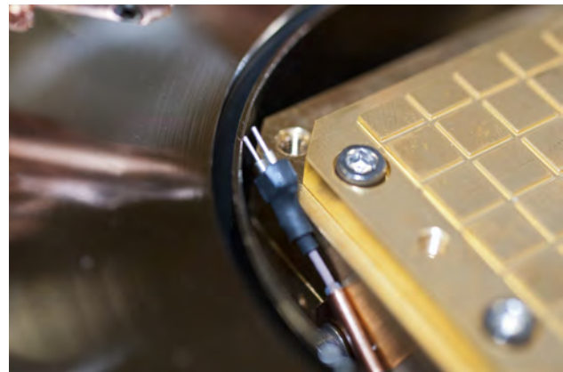
FIGURE 4-4 Left: Disconnecting the triaxial sample holder; Right: Cable plug left out after disconnecting
