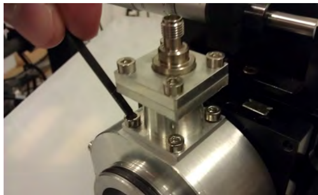
FIGURE 5-15 Remove the bottom set of four M3 screws
