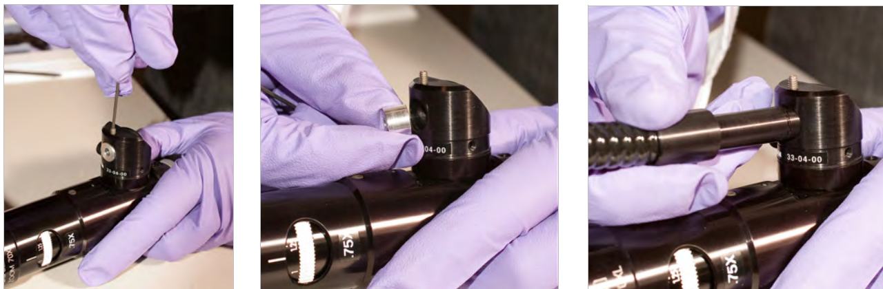
FIGURE 3-25 Left: Loosen the set screw on the fiber optic cable fitting; Middle: Remove protective fitting; Right: Insert the fiber optic cable
