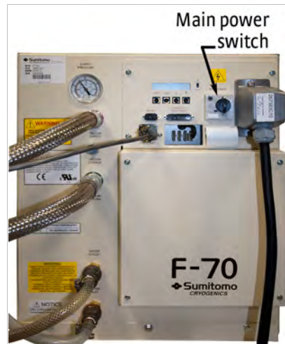
FIGURE 4-10 CCR compressor panel
