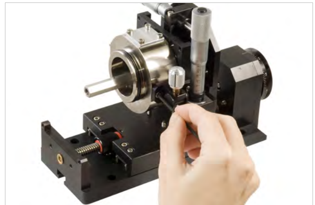
FIGURE 5-24 Left: Thread the shaft through its mounting hole; Right: Attach the planarization assembly to the probe arm base
