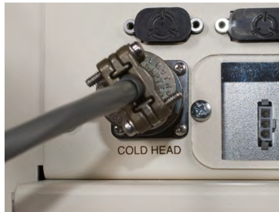
FIGURE 3-16 Left: Connect the cable to the cold head; Right: Connect the cable to the compressor
