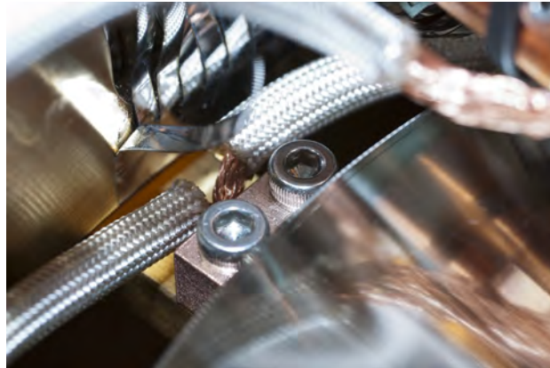
FIGURE 3-33 Braid block mounted to the radiation shield
